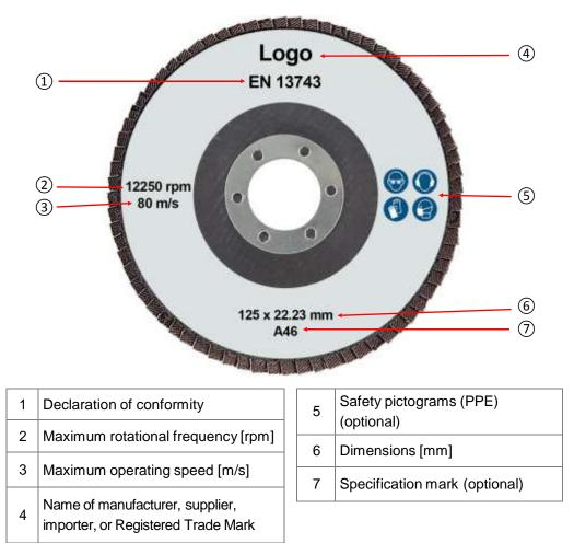
\* EN 13743 marking shows that the producer has followed the essential safety requirements of the European safety standard for flap discs in order to reduce the risks for the end-user.
